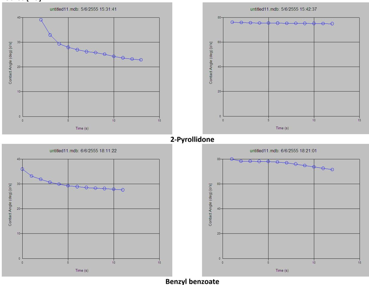
Fig. 1 Contact angle variation with time of different solvents (left: on glass and right: on PDMS)
