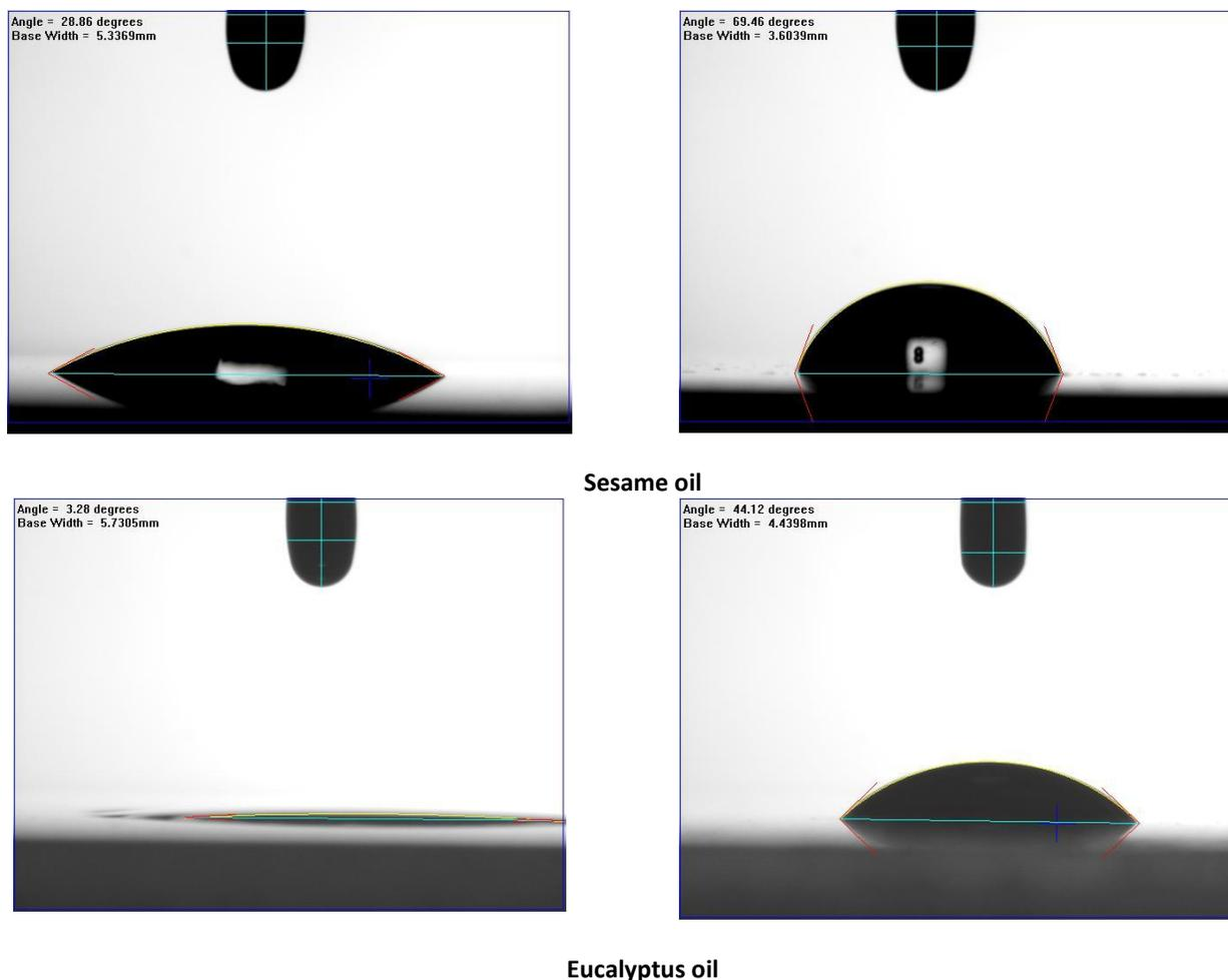
Fig 2: Contact angle of different solvents (left: on glass and right: on PDMS) (continued)
